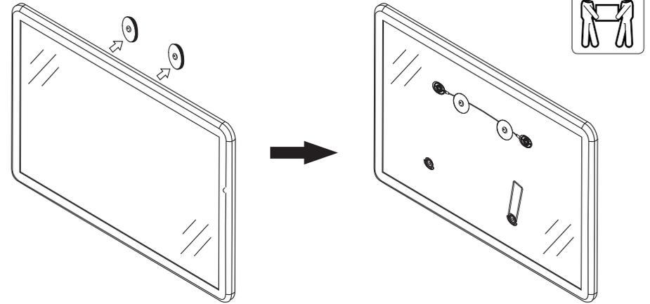
After the wall mount has been safely secured to the wall, Carefully lift your TV and hook wire rope into the wall plate rail. Make sure your TV is securely and correctly attached.
