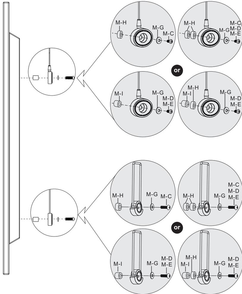
**Note:** Choose the appropriate screws, washers and spacers (if necessary) according to the type of screen.
