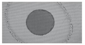
A connector with a dry residue that needs cleaning.
