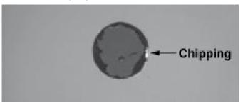
A connector with damage to the cladding. Cleaning cannot remove damaged cladding. A small amount of epoxy around the cladding is allowable, but this shows excessive epoxy around the cladding that does not clean off. This connector must be replaced.
