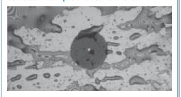
A connector with liquid or oil contamination that needs cleaning.
