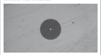
A connector with an oil residue that needs cleaning.
