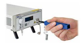
1. Remove the guide cap completely from the device, and insert the tip of the tool into the optical port connector. Push the case to start the cleaning process; a click indicates that the cleaning is complete. 2. Insert optical cable
