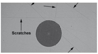
A connector with scratches. These scratches are not detrimental to the endface and does not clean off. But, deep scratches that appear to cross the fiber-optic core can cause signal loss.
