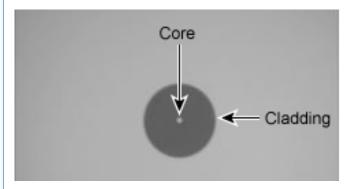
A clean connector should not have any major debris or scratches across the core.
