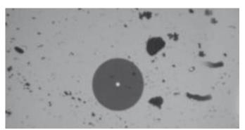
A connector with dust particles spread across the surface of the endface that needs cleaning.
