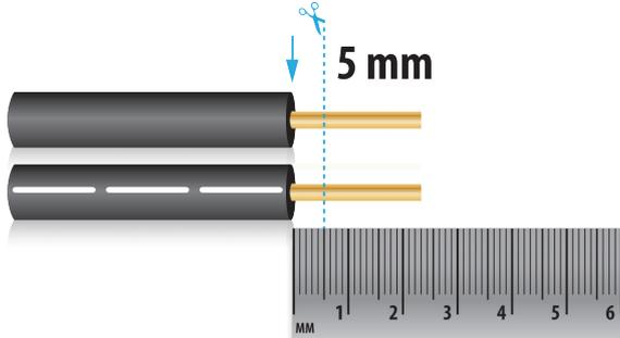
The captive screw plugs for power, RS-232 and contact controls are supplied with the unit. Separate the wires about 2,5cm long; strip off precisely 5mm of the wires insulation from the end.
