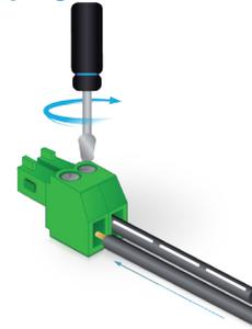
Identify the positive and negative leads of the power supply before assembly. When using a 3rd party PSU this must be checked before assembly. **CAUTION - always confirm your PSU connection with a multimeter before inserting it into the product - a miswired connection will cause damage to the product and void the warranty!!**
