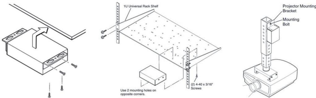
The under desk mount is sold separately (LU-UDM-100); the product also fits many other mounting hardware from Extron, Middle Atlantic, etc. Only use the type 4-40, 3/16" (5mm) long screws supplied with the mounting hardware to screw onto the product. Wrong type of screw
