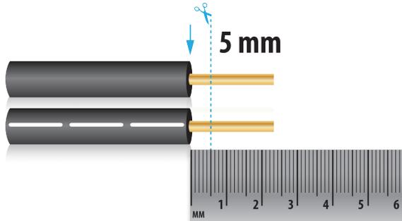
The captive screw plugs for power, audio, RS-232 and contact controls are supplied with the unit. Separate the wires about 1" (2.5 cm) long; strip off the wire insulation precisely 3/16" (5mm) from the end.
