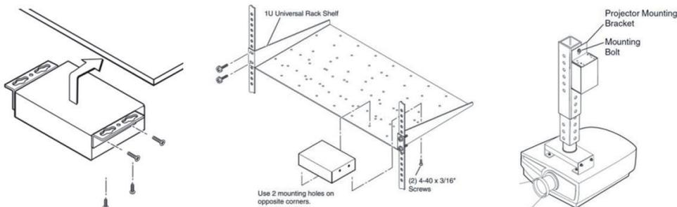
Luxi has the under desk mount sold separately (Luxi P/N 78-002-01); the product also fits many other mounting hardware from Extron, Middle Atlantic, etc. Only use the type 4-40, 3/16" (5 mm) long screws supplied with the mounting hardware to screw onto the product. Wrong
