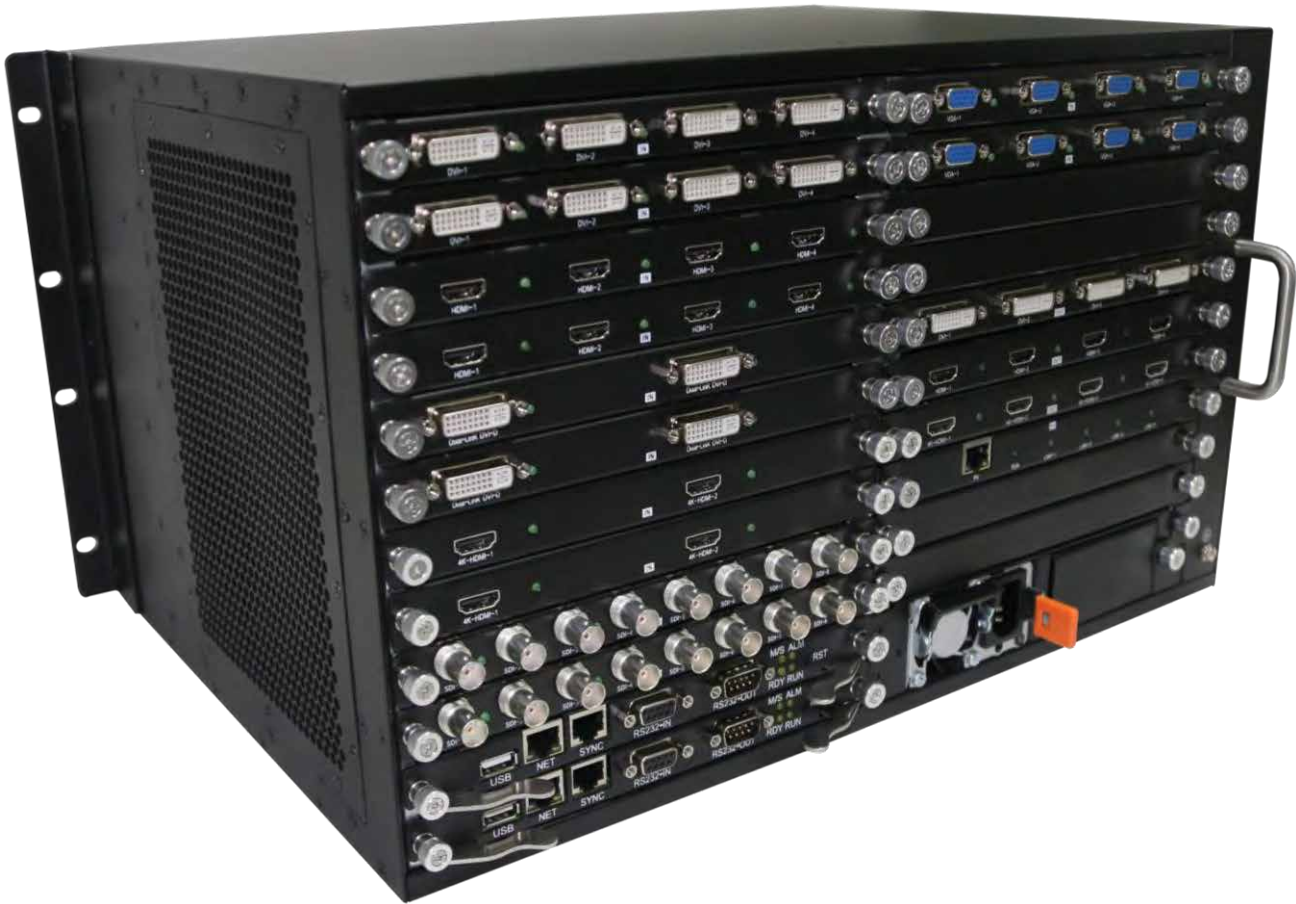
DB-VWC2-C6 Rear view with twelve input cards, three output cards, one network previewing card, and two control cards
