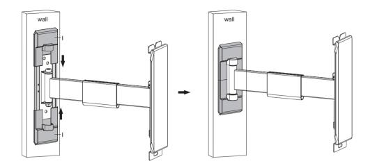
Note: Pull the articulated arm and make it vertical to wall ,insert both top and bottom plastic covers
