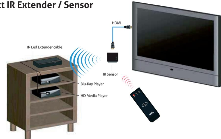
Plug the IR LED Extender cable into the IR OUT connector of the WHD100-V2 Transmitter. Attach the IR LEDs to the front of your HD devices. This will now send all received infrared commands via the IR Sensor of the WHD100-V2 Receiver.
