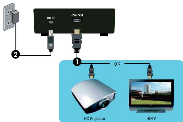
1. Connect your HDTV or HD Projector (HDMI IN) via an HDMI cable to the WHD100-V2 Receiver (HDMI OUT).
