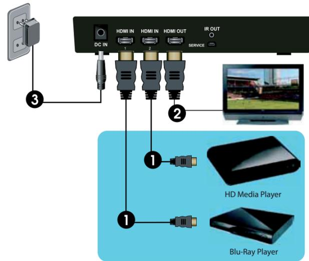
1. Connect max. 2 HD devices (HDMI OUT) via HDMI to your WHD100-V2 Transmitter (HDMI IN).
