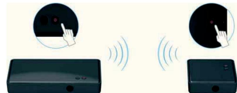
1. If the WHD100-V2 is in Standby mode (red POWER LED), press the ON/OFF button of the WHD100-V2 Transmitter and Receiver to switch them on. It takes about 80 seconds for the system to start up.
