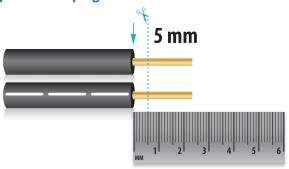
The captive screw plugs for power, RS-232 and contact controls are supplied with the unit. Separate the wires about 2,5cm long; strip off precisely 5mm of the wires insulation from the end.
