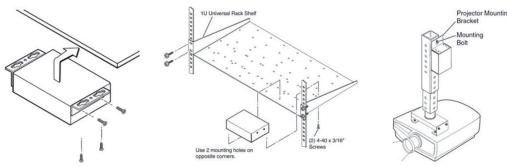
The under desk mount is sold separately (LU-UDM-100); the product also fits many other mounting hardware from Extron, Middle Atlantic, etc. Only use the type 4-40, 3/16" (5mm) long screws supplied with the mounting hardware to screw onto the product. Wrong type of screw
